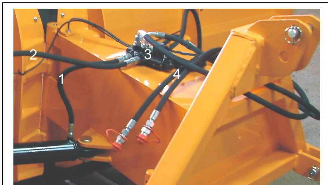
Fig. 12 Variable geometry double-blade wheeled snow plough - hydraulic supply elements
